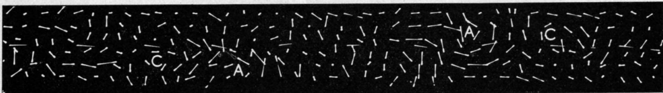
Fig. 6. Oscillograms showing wind fluctuation vectors produced as eddies pass through a cross-wind line. (a) 1600 GMT 15 May 1963, line 12,5 m, longitudinal scale 1.2 sec per row, wind speed 4.5 m/sec -1 . (b) 1245 GMT 5 March 1964, line 30 m, longitudinal scale 1.8 sec per row, wind speed 6 m/sec -1
